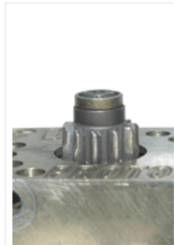
A Worn & Broken Gear Teeth (side)
