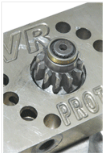
A Worn & Broken Gear Teeth (front)
