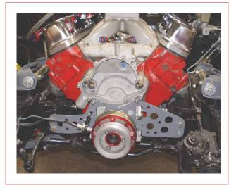
Check the drive shaft angle to make sure it is straight at the u joint. When you have it set as to where the motor will be, take small blocks of steel and place one under each end of the plate as a stop to rest the motor mount on. Angle iron will also work. Weld this in place. Take the chain hoist off the motor and check the alignment again.
